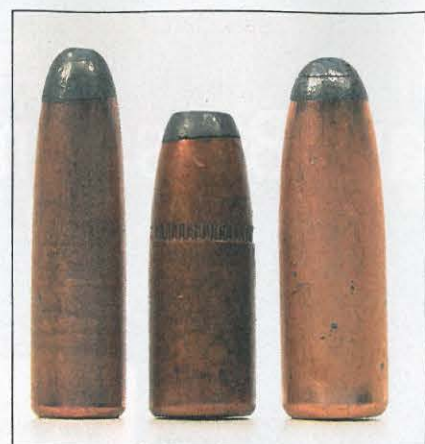
Hawk bullets include (left to right): a 160-grain, .286-inch semi-roundnose; a .32-caliber (.321-inch) 170-grain flatnose; and an 8mm (.323-inch) 200-grain roundnose. The .32 is especially useful because its cannelure is in the correct place for the .32-40.
