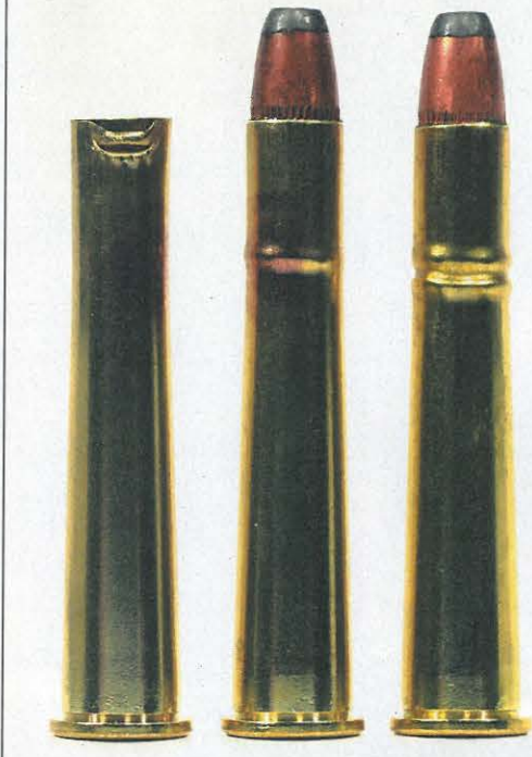
The .32-40's straight tapered case can be tricky to load. Carefully condition and bell case mouths, even when loading jacketed bullets; a slightly longer case or incomplete cannelure can ruin brass.
